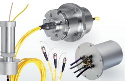
High-definition video signal transmission of HD-SDI signals (1080P, 4K) with up to 3GHz high-frequency. Advanced fiber-brush technology and gold-to-gold multi-contacting for high contact guality and low resistance. Customized, combined power and signal versions possible.
