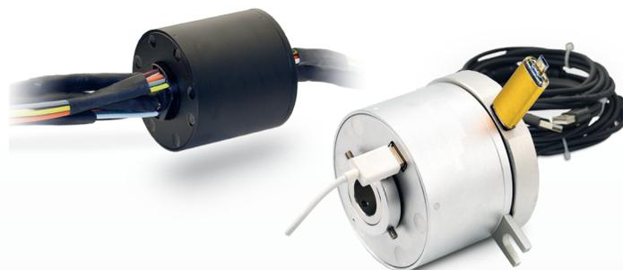
Hybrid sliprings for USB and electrical power/signals transmission. USB1.0, USB2.0 and USB3.0, USB3.1, USB3.2 transmission up to transmission rates of 20Gbit/s. Capsulated or through-bore housing design for individual implementation. Standardized and modularized design.
